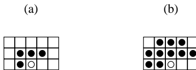
Fig. 1. Two examples of causal context neighborhoods. Solid dots indicate conditioning pixels, while the unfilled dots indicate the pixel currently being encoded or decoded.
