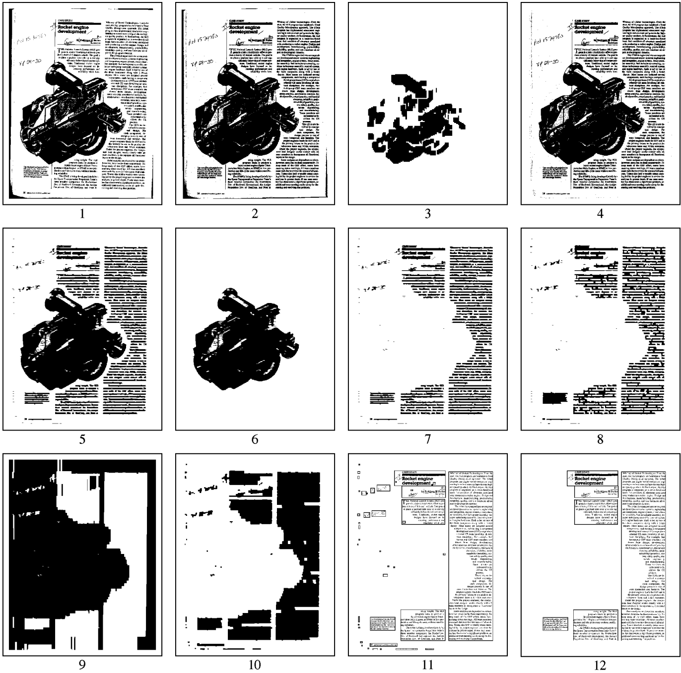
Figure 3: Early segmentation. The input image (1) is deskewed (2); a mask (4) is thickened to (5), then filled from the seed (3) to form the half-tone mask (6). This is subtracted from (5), leaving (7), which is slightly dilated (8). The vertical whitespace mask (9) is constructed and subtracted from a considerably dilated version of (8), leaving a proto-textblock mask (10). These regions (11) are then sieved to remove noise and graphics (12).
